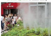
Low-cost cooling system with Semi Dry Fog®, which provides effective evaporative cooling effect without wetting people.
